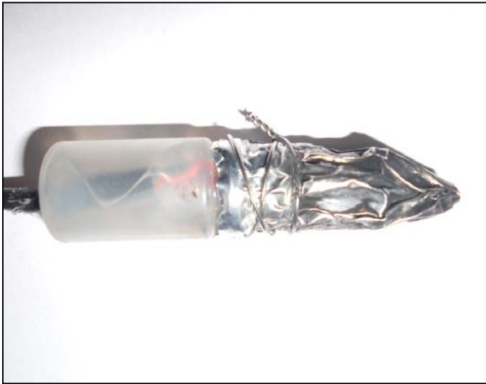
Fig.11 Temperature Sensors: LM35 and NTC. The sensors are protected from damage by using sparkles which were glued to aluminium foil.
